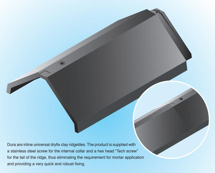
The ridgetile is produced by one of Europe's largest and most innovative clay rooftile manufacturers, based in Portugal. The Dura Ridge System was designed to consider Irish weather conditions such as the frequency of very high winds. Traditional bedded (mortar) ridges can be subjected to loss of tiles in gales, particularly the end tiles facing edge-on to the wind. Dura ridge can withstand such weather conditions because of the simple but robust fixing method.
